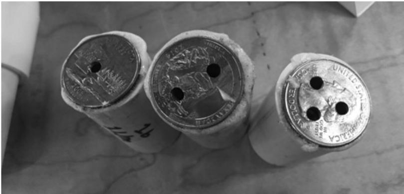
**Figure 6:** The three different flow restrictors. A 2-inch long piece of PVC is glued to a quarter with the proper number of  $\frac{9}{64}$ -inch holes. Each hole allows 1 liter to flow per minute so the leftmost flow restrictor is 1 liter per minute, the middle is 2 liters per minute and the rightmost is 3 liters per minute.
