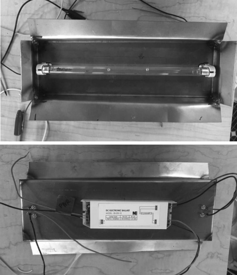
Figure 10: Top of the reactor chamber fully constructed (not attached to power source).
