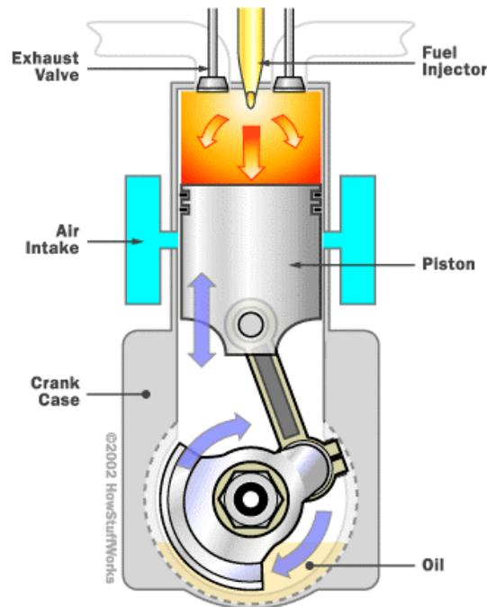
Figure 5. Shows the main components of a diesel engine piston. This figure is specifically of a two-stroke piston. It is important to note that diesel pistons only compress air as opposed to gasoline pistons, which compress a mixture of gas and air (HowStuffWorks, 2008).
