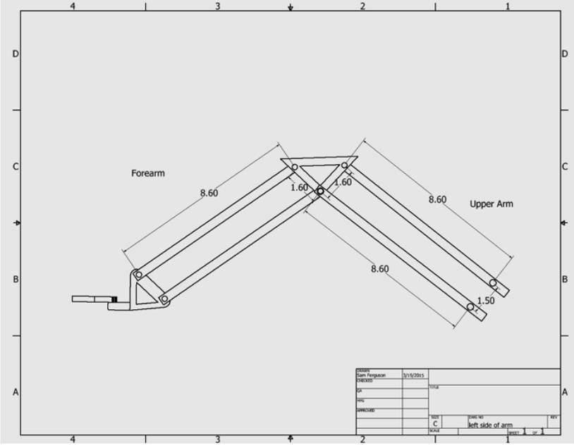
Figure 7: The left side of the robotic arm (dimensions in inches).
