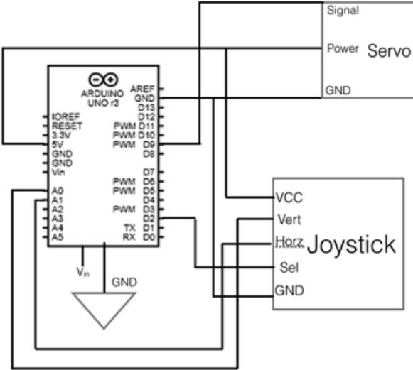
Figure 9: A sample circuit diagram for a single servo controlled by an Arduino Uno and a joystick. See Appendix for code.
