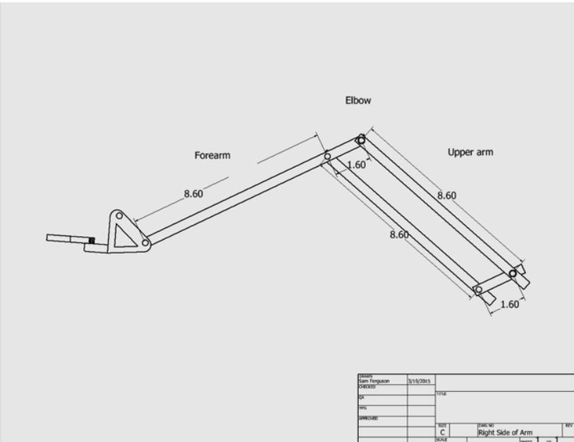
Figure 8: The right side of the robotic arm (dimensions in inches).
