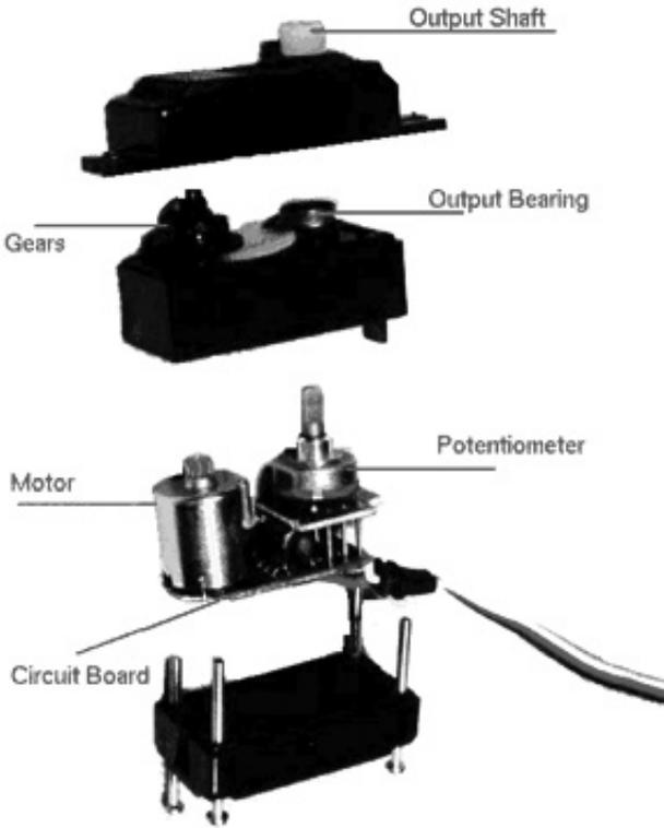
Figure 10: The inside of a servo motor [7].
