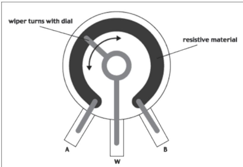
Figure 11: *The inside of a potentiometer [8].*
