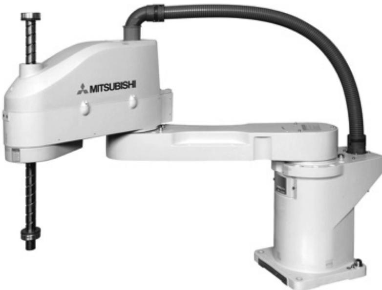
**Figure 2:** *A Sample SCARA Industrial robot [4].*
