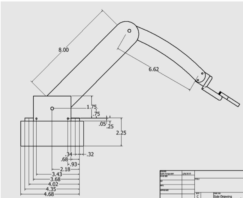
Figure 4: Side view of CAD drawing of the version 1.0 (dimensions in inches).
