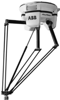
**Figure 1:** A Sample Delta Industrial robot [3].
