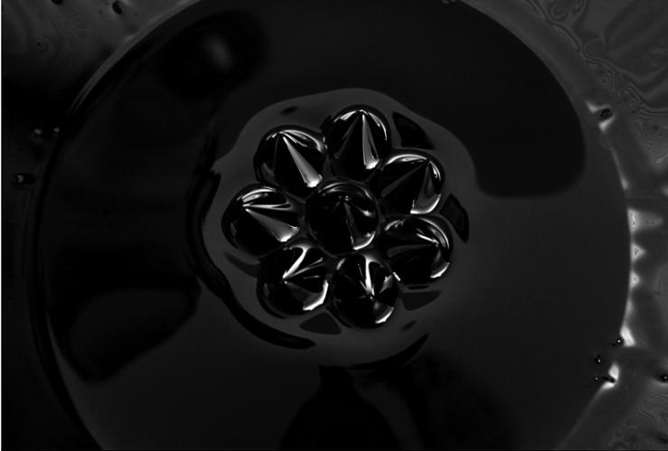
**Figure 2:** A small number of large spikes are formed when the magnet is distant.
